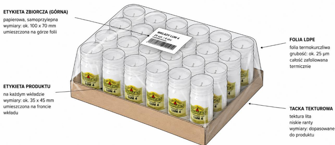
Figure 2. Illustrative configuration of the bulk packaging for inserts
